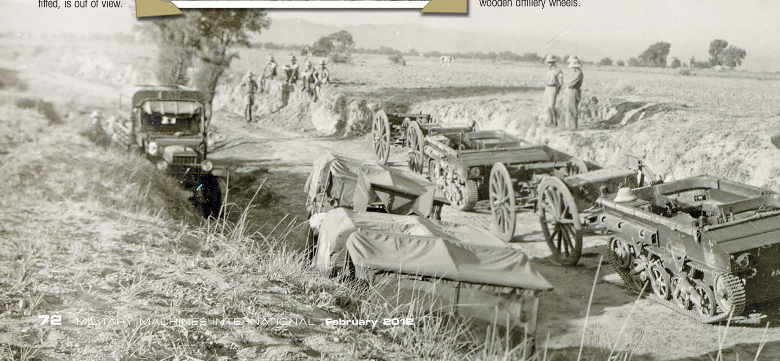
Right: Mk IIC Light Dragon negotiates some rough terrain, with what looks to be a limber of the type used with the 4.5 in howitzer in tow, although the gun, if fitted, is out of view.
