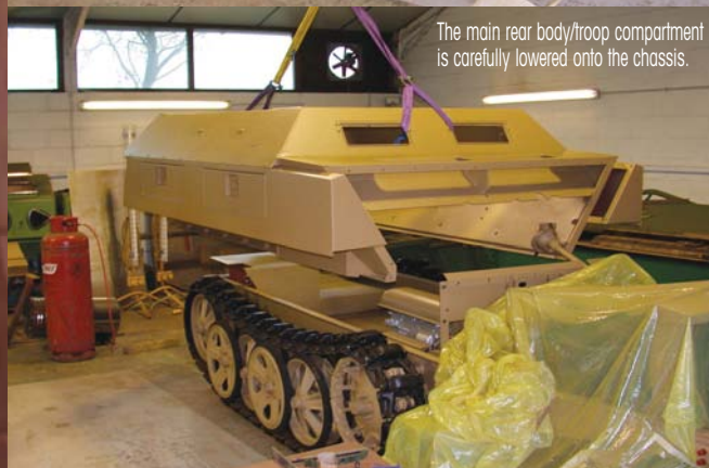
With the lower hull/chassis in the background, here we see the two main armoured components waiting to be fitted.
