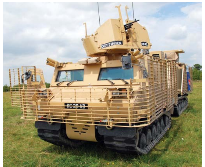
Above: Warthog is the British Army's new All-Terrain Tracked Carrier and will be operated by the Queen's Royal Hussars who are normally based in Athlone Barracks, Sennelager. It was developed by Singapore Technologies Kinetics Ltd and modified by Thales to meet British Army requirements.
